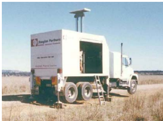
Figure 2: Purpose built CPT rig
